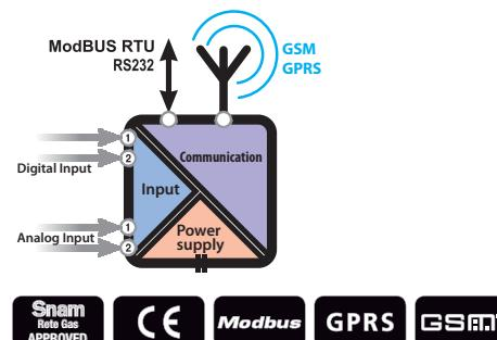
M-RTU-PC is a specific monitoring solution for cathodic protections: monitoring of parameters and analysis of material corrosion (oil and gas pipelines, tanks, plants, buildings, docks, etc.). The low power consumption allows also a battery power supply (3 years life-time). M-RTU-GP is able to acquire, process, store and transmit analog or digital signals to a PC central station using GSM and GPRS standard communication.
